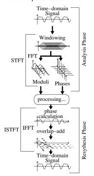
Figure 1. Phase-Vocoder functionality
