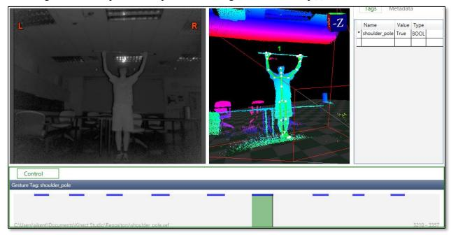
**7.** After you have finished tagging all of the appropriate portions of the clip(s), right click on the solution and hit "build". This will provide the .gbd file that will be uploaded to the website.
