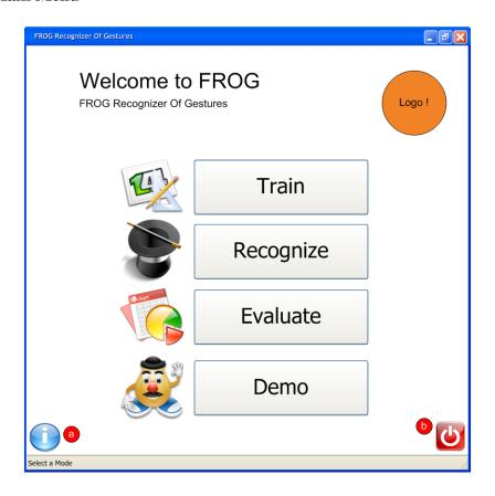
This is the main window of the program. From this window the user can access the different modes. In order for this window to display, it is necessary for the system to find at least one device plug-in to work with. If no plug-in is encountered, then the program will ask the user to install a plug-in.
